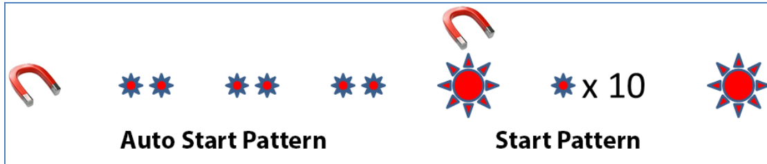
Figure 7—Magnet and indicator light sequence to switch from Auto Start to Start. A magnet swipe near the communications port, will double-blink three times. Then the indicator light will remain on for two seconds. Swiping the magnet again in the window while the light is on will put the tag in Start mode. The tag will blink 10 times rapidly and then remain lit for two seconds to show it is activated.
