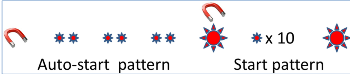
Figure 4 - Magnet and indicator light sequence to switch from Auto Start to Start. After an initial swipe of a magnet near the communications port, the indicator light will show a double blink 3 times when in Auto Start. Then the indicator light will remain on for 2 seconds. Simultaneously swiping the magnet again with the light on will Start the tag. The tag will blink 10 times rapidly and then remain lit for 2 seconds to show the tag is Started.
