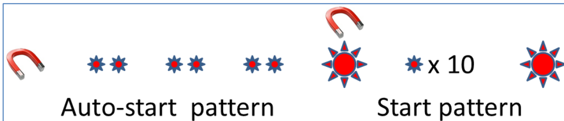
Figure 3 - Magnet and indicator light sequence to switch from Auto Start to Start. After an initial swipe of a magnet near the communications port, the indicator light will show a double blink 3 times when in Auto Start. Then the indicator light will remain on for 2 seconds. Simultaneously swiping the magnet again with the light on will Start the tag. The tag will blink 10 times rapidly and then remain lit for 2 seconds to show the tag is Started.
