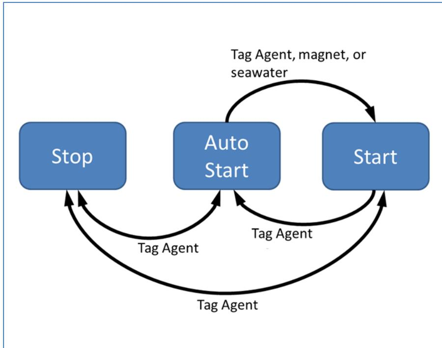
Figure 3 - Methods for changing a SPOT-325 tag's state.
