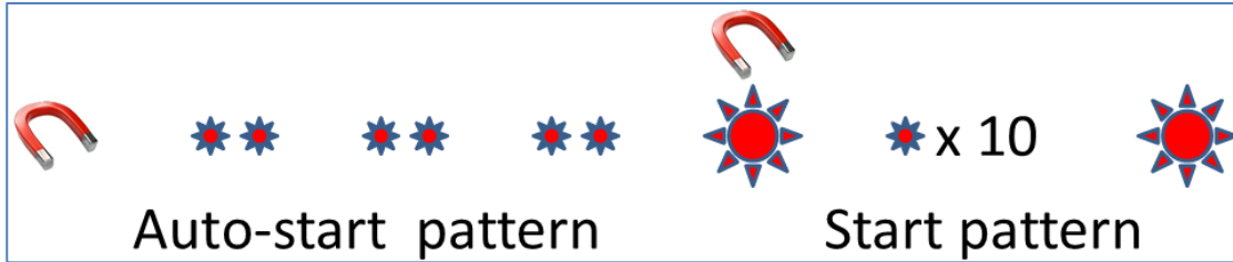
Figure 4 - Magnet and indicator light sequence to switch from Auto Start to Start. After an initial swipe of a magnet near the communications port, the indicator light will show a double blink 3 times when in Auto Start. Then the indicator light will remain on for 2 seconds. Simultaneously swiping the magnet again with the light on will start the tag. The tag will blink 10 times rapidly and then remain lit for 2 seconds to show the tag has started.
