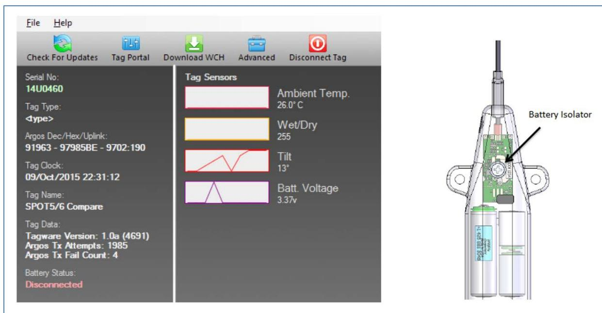
Figure 22—Tag Agent showing the Battery Status as disconnected and the placement of the battery isolator screw on a SPOT-F-257 tag
