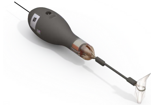
Figure 1—sPAT tag rigged with a stainless-steel heat shrink-covered tether and a Wilton anchor
