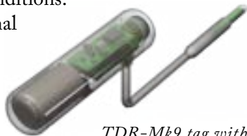
TDR-Mk9 tag with optional sensor stalk, designed for implantation
