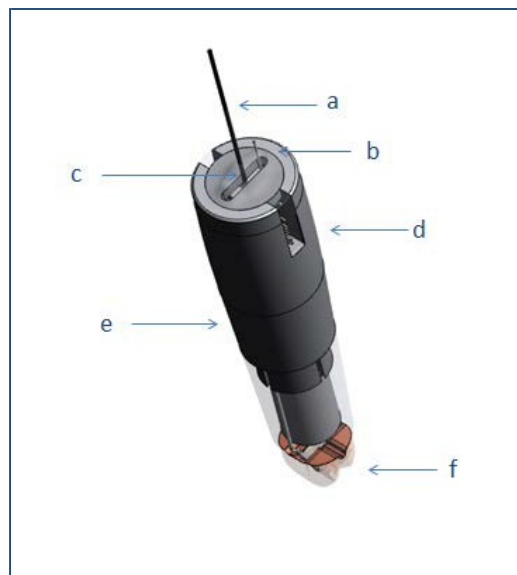
Figure 1—mrPAT tag showing: (a) Argos antenna, (b) wet/dry sensor, (c) LED indicator light, (d) communications port, (e) float, and (f) release pin.
