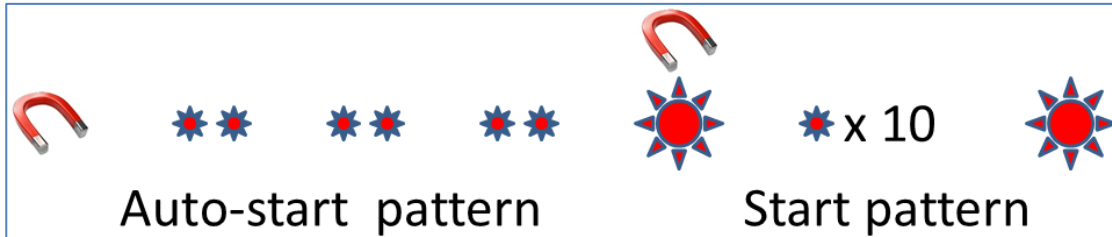
Figure 2—sample of the indicating light pattern
