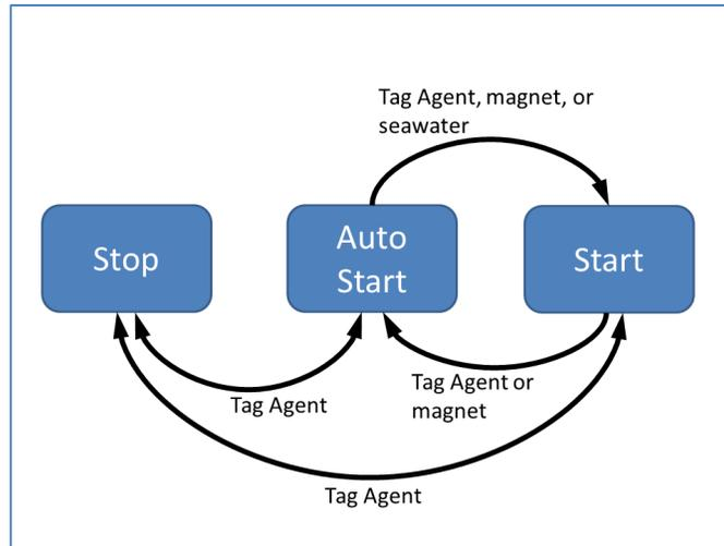
Figure 3—methods for changing a SPOT-F state. Tag Agent can be used to put a SPOT-F in any state.
