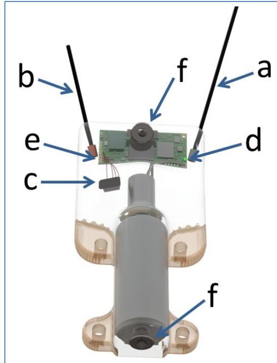
Figure 1 -A typical SPOT-F tag showing the Argos antenna (a), Fastloc® GPS antenna (b), communications port with plug (c), indicator light (d), magnetic switch (e), and wet/dry sensor (f)
