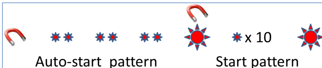
Figure 2—sample of the indicating light pattern
