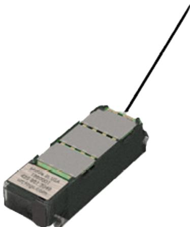
**Argos antenna**—minimally intrusive, low-lying antenna exiting the rear of the tag is lightweight, highly robust yet super flexible. The antenna is securely anchored in epoxy resin and withstands over 100 pounds of tensile force ensuring it will stand up to abuse from birds.
